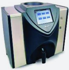
GRAIN Moisture ANALYSIS DICKEY-JOHN GAC 2500-UGMA Moisture Range: 5 to 45% (grain dependent)
