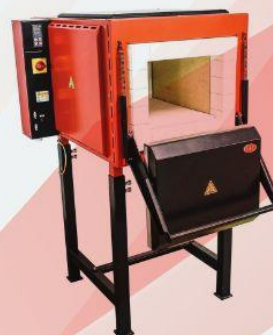
PKE Hardening chamber furnace up to 1,280 °C (12.2-87 Liters)
